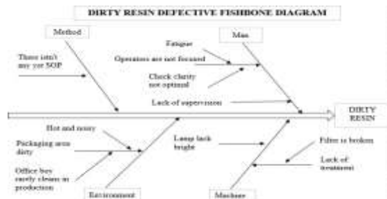
Figure 3. Fishbone Dirty Resin Defects (Source: Data Processing, 2022)
