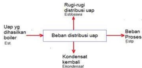
Figure 7. Energy balance in distribution load
