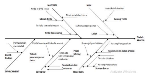
Figure 3.2 Diagram of the Cause and Effect of Defective Products
