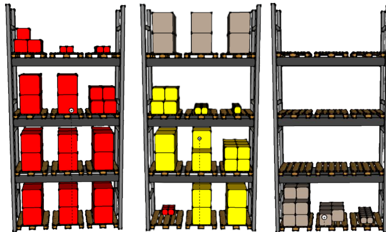
Figure 6. The location of the center of mass on each shelf using First Algorithm
