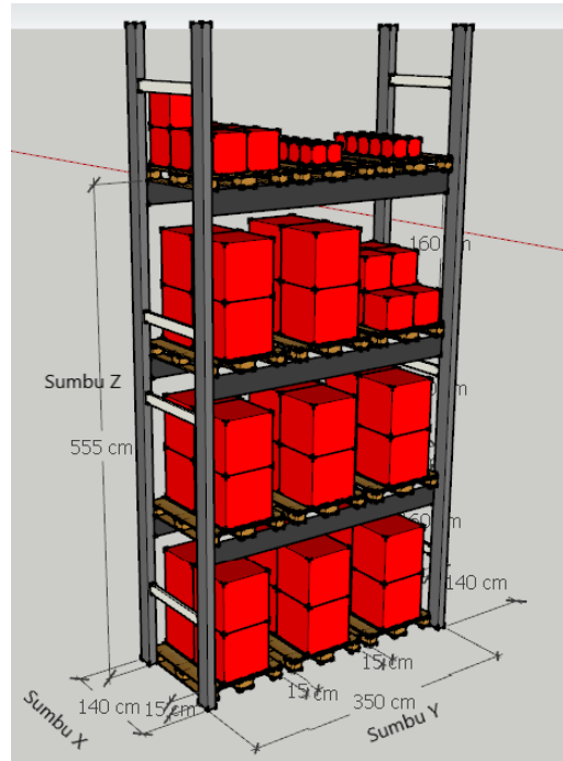
Figure 5. Pallet placement illustration for each layer on the first shelf.
