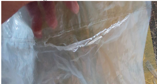
Figure 3. Detached Seal Defect
