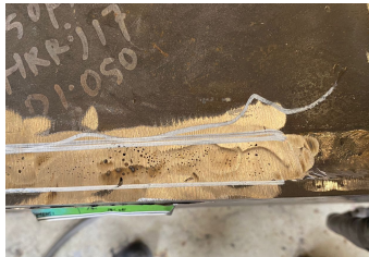
Figure 2. Porosity defect (source: PT. INKA Multi Solusi)
