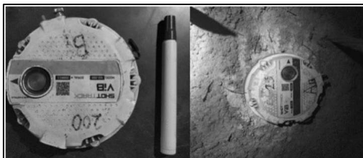
Gambar 4. Alat Monitoring PPV, (Sumber: PT.FI)
