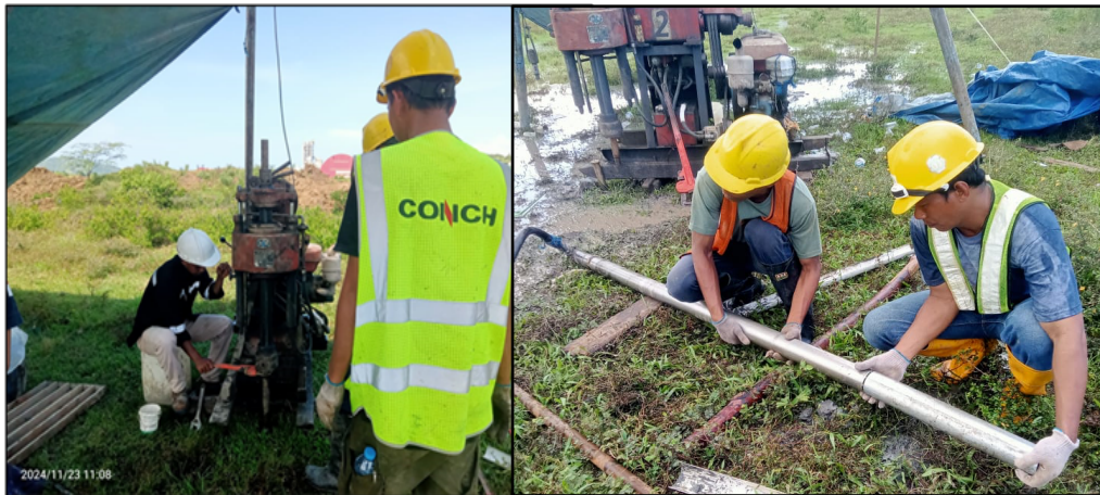
Gambar 2. Kegiatan pengambilan Sampel UDS ( Undisturbed Sample )
