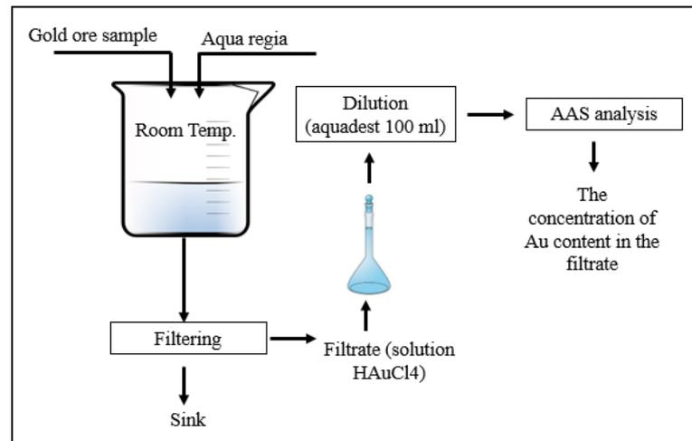
**Figure 2.** Design of leaching process
