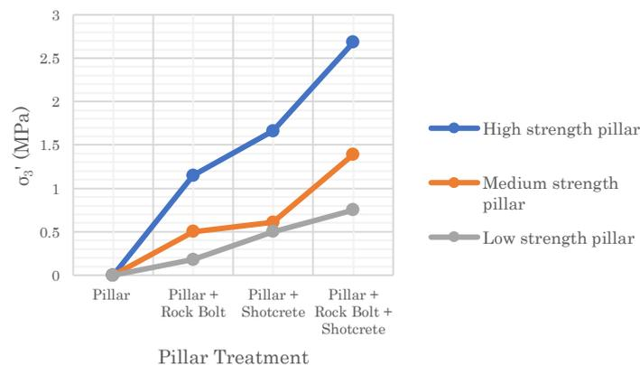
**Figure 11.** Equivalent confining pressure on each pillar
