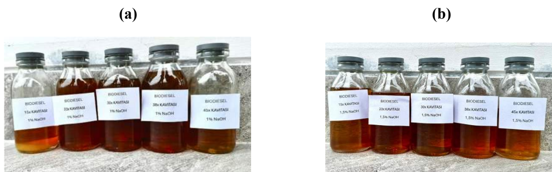
Figure 3. Visual characteristics of the biodiesel produced in this study: (a) Biodiesel sample with 1% NaOH concentration; (b) Biodiesel sample with 1.5% NaOH concentration.
