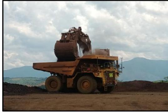
Gambar 1. Proses *Loading Slag* Nikel ke *Haul Truck*
